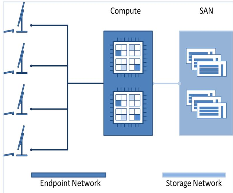
Figure 1. Basic VDI implementation using separate Compute and Storage components
