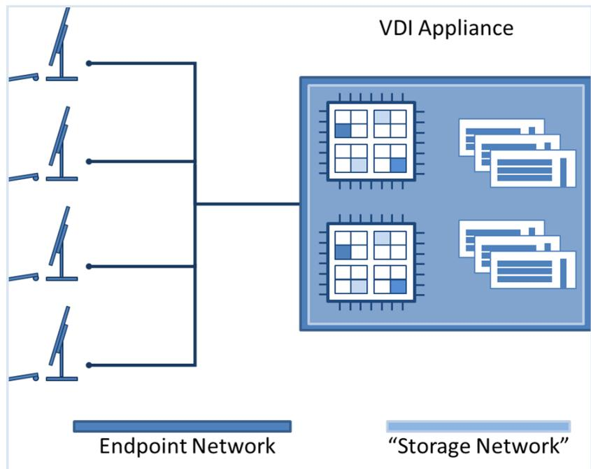
Figure 2. VDI appliance with integrated Compute and Storage components
